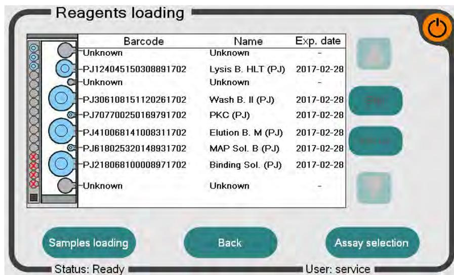
**Figure 6:** “Reagent-loading” screen of the InviGenius® software
