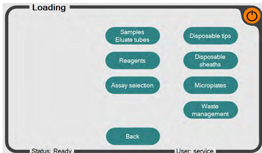
**Figure 4:** Loading screen of the InviGenius® software
