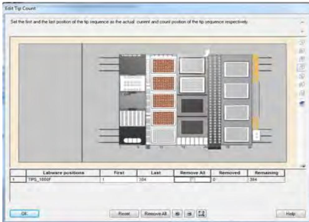
Please ensure that the loaded filter-tips are shown at the right position of the picture. If not, this has to be adapted/ modified on the computer.
