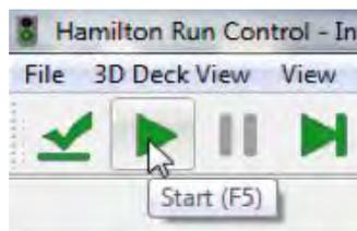
The machine will initialize and start a dialog prompting how many samples will be processed. It is necessary to use a multiple of 8 samples. In case of different numbers of samples, please complement to 8 with water samples.
